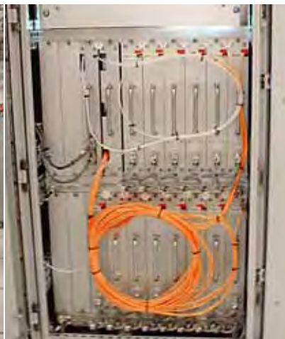
Open laser chassis displaying the modular design of high power fiber lasers
