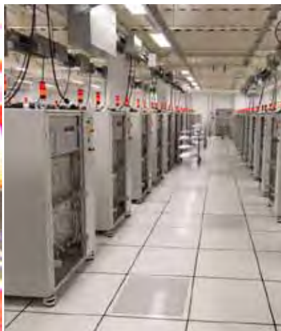
Diode burn-in facility
